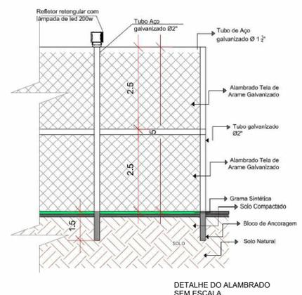
DETALHE DO ALAMBRADO SEM ESCALA
